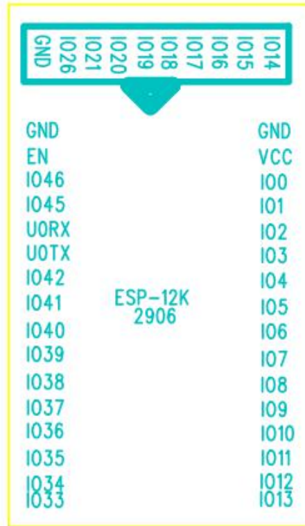
ESP-12K PIN definition diagram
