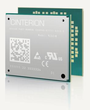
Cinterion® PLS62-W Wireless Module Global Connectivity with Multi Band LTE Cat 1 and 2G / 3G Fallback
