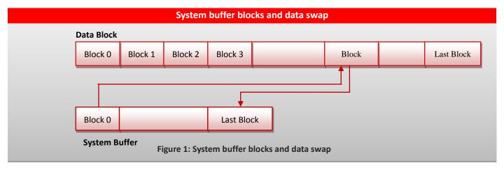
In the worst case scenario the host keeps writing data to Block N while the system buffer blocks are used frequently and the other data blocks are not used at all. All system buffer blocks would be worn out after around
