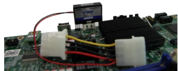
Figure 1: SATA with cables
