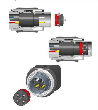
Insert Sleeve Holder "A" in Connector Body "B" with red side inside connector.
